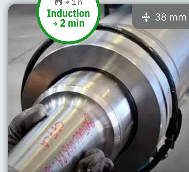
STEEL TUBE SHRINK-FITTING - FRETAGE DE TUBE ACIER Inductor L180/D300 (on demand) Powerduction 220LG
