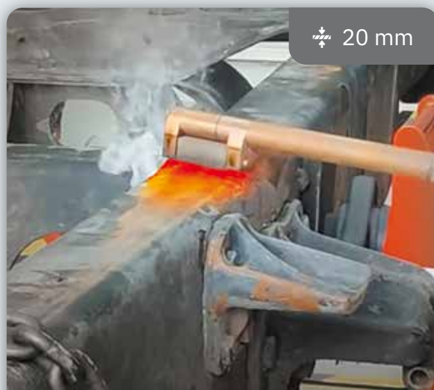
TRUCK CHASSIS STRAIGHTENING - REDRESSAGE CHASSIS DE CAMION Inductor L90 Powerduction 220LG
