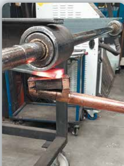
TRAILER MANUFACTURE - STEEL BENDING - FABRICATION DE REMORQUE - CINTRAGE ACIER Inductor L70 Powerduction 220LG
