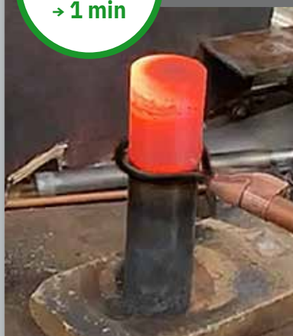
STEEL BAR FORGING - FORGEAGE BARRE ACIER Inductor L180/D60 Powerduction 220LG
