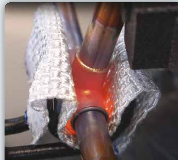
BRAZING COPPER FITTING - BRASAGE RACCORD CUIVRE Inductor L90 Braz 28 Powerduction 110LG
